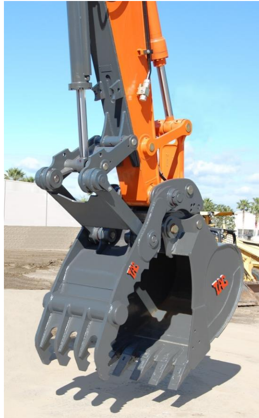
Main-Pin Hydraulic Thumb With Unitized Links and Cylinder Assembly
