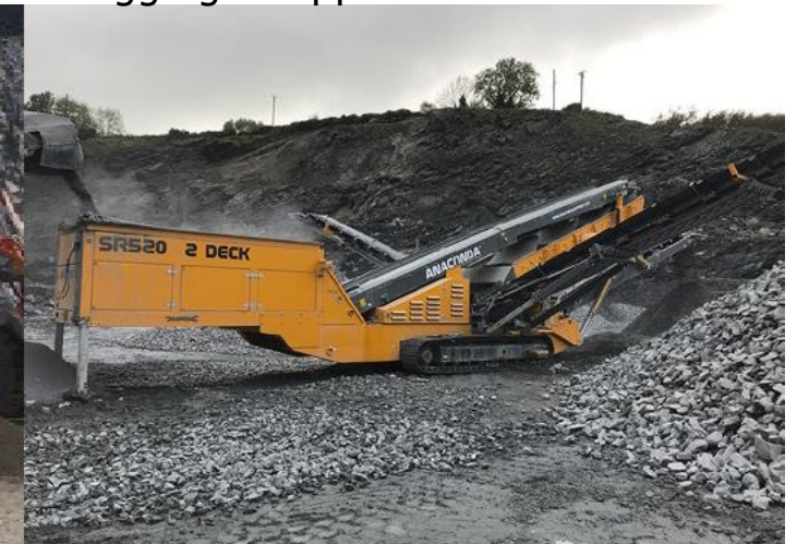
SR520 (2 Deck) working in a Quarry application in Ireland.
