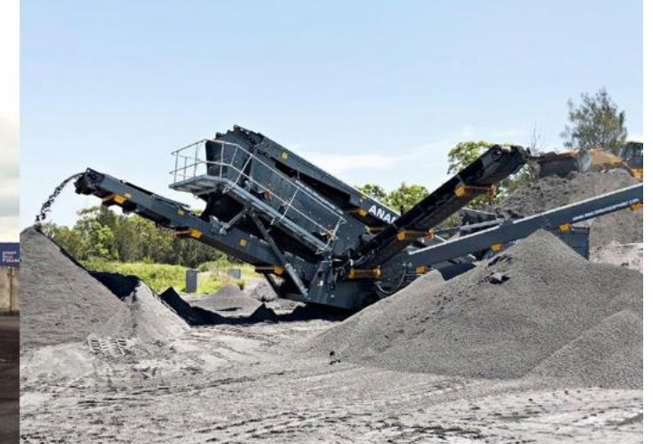
SR514 (3 Deck) working in an Aggregate application in Australia.
