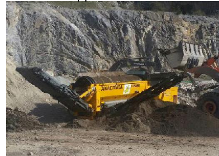
TD516R Trommel Screen working in a Compost application in Austria.
